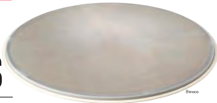
FIGURE 1. Sweco Fusion screens eliminate the use of adhesive, epoxy or silicone in screen manufacturing. Instead, the mesh is fused directly to the polymer tension ring
