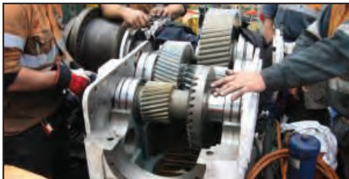
FIGURE 2. Disassembly of a gear unit for inspection allows operators to inspect gear-contact patterns after installation or during operation. Under ideal conditions, the contact pattern across each tooth will be uniform around each gear (indicating full contact). However, machining, assembly errors, distortion of the gear unit housing and misalignment can create problems. An improper gear-set contact pattern creates high stresses on the gear teeth
