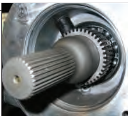
FIGURE 7. Continuous (online) vibration monitoring should be implemented for critical gear units. The dynamic forces and vibration that result from gear meshing often present challenges to unit reliability, causing excessive gear and bearing wear and adversely affect the driver, driven equipment, steel structures, foundation and even nearby equipment
