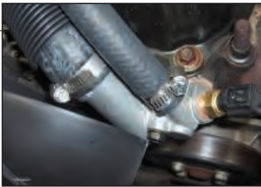
FIGURE 5. The root cause of rotating machine component failure is often found in the supporting auxiliary system, particularly the oil or cooling systems. Since change in the coolant supply temperature is a common cause of many machine failures, coolant temperature sensors (shown here) should be used
