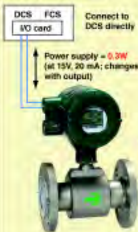
FIGURE 1. Four-wire mag meters are better for heavy-slurry applications. Two-wire mag meters do not require separate wiring to a power source.
